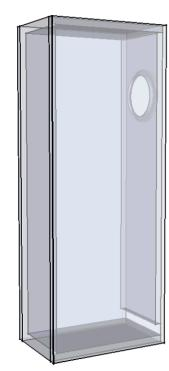
o/ drawing uses 3/4" (19.1mm) material. 18-20mm OK. Quality multi-ply recommended 1/ stuff with 0.75 lbs / ft^3 (1.59 pounds = 0.72 kg) of polyfill 2/cleats on back to allow for removable back, useful for adjusting the stuffing
