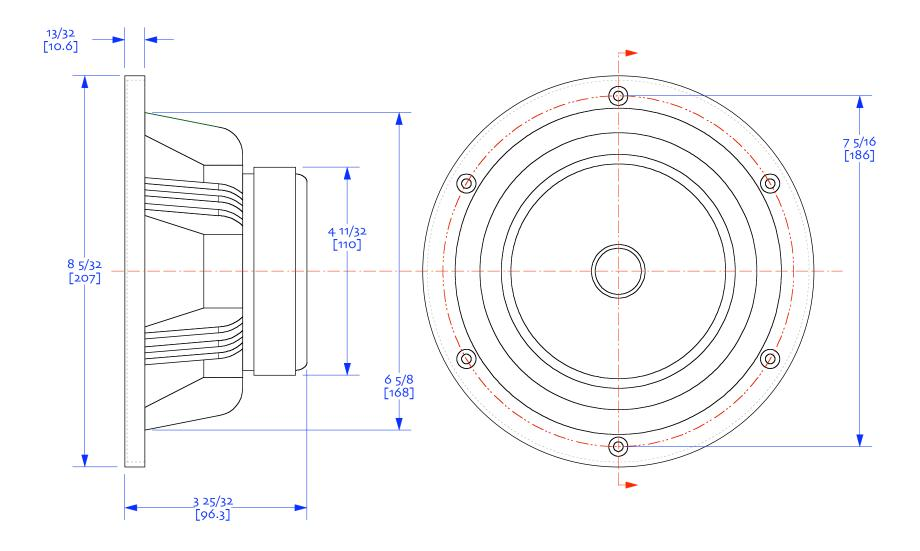
Gasket is 2 mm thick uncompressed, 1.5+mm compessed
