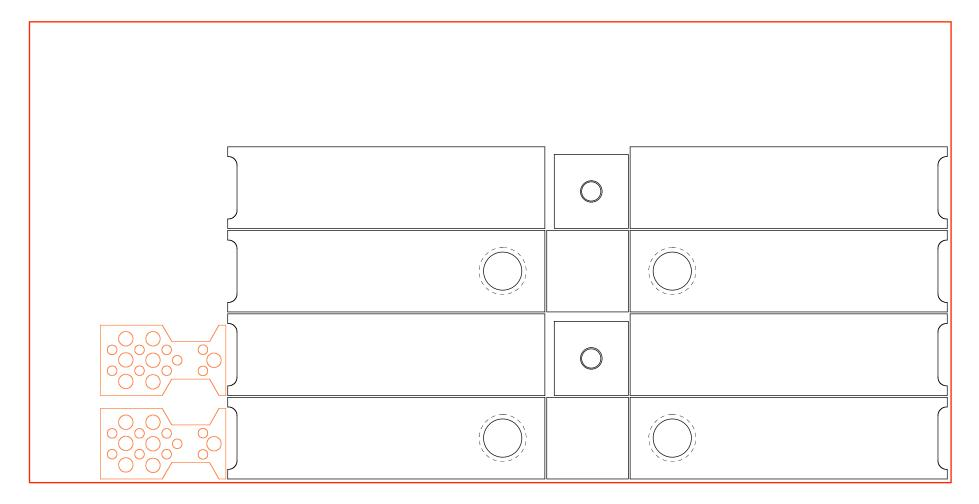
1) The plans attached are for maximum yield, and include kerf and trim cut allowances for our production saws (5mm and 10mm respectively) that DIYers could reduce, but without significant effect on the yield or pattern.
