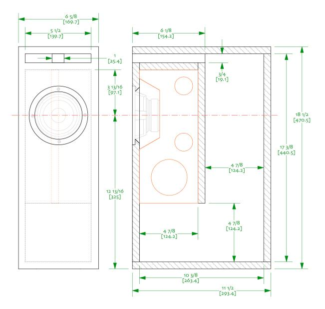
o/ All panels 15mm (5/8") thick. Dimensions shown to 1/16" and 0.1 mm but need not be built to that accuracy.
