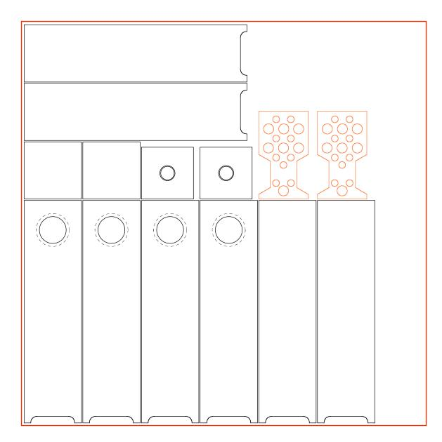
1) The plans attached are for maximum yield, and include kerf and trim cut allowances for our production saws (5mm and 10mm respectively) that DIYers could reduce, but without significant effect on the yield or pattern.
